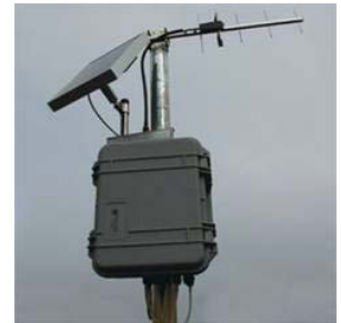
Telemetry for the leak detection project
