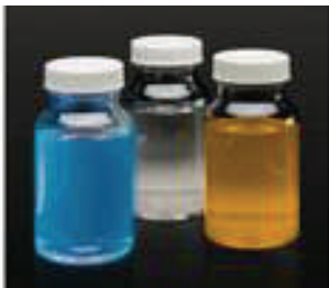
Selective substrates in Colilert media change colour and fluoresce in the presence of different bacteria
